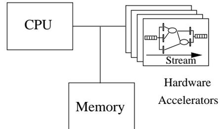
Figure 1: A computer system with hardware accelerators such as Stream Architectures.
