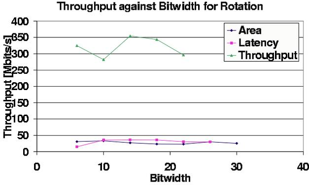
Figure 7: Bitwidth / Throughput tradeoff.
