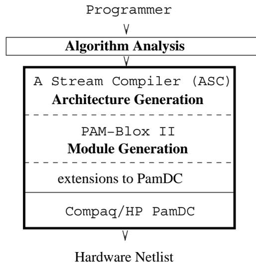
Figure 2: Levels of abstraction and structure of ASC. The bold box represents a single C++ program.
